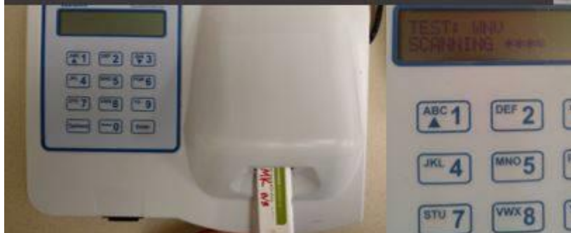
Steps 6, 7: Insert into RAMP tester and record
