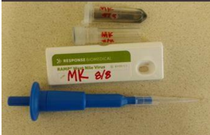
Steps 6, 7: Insert into RAMP tester and record
